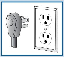
cord. Do not use a power cord that is frayed or damaged. The use of a ground fault interrupter (GFI) is not recommended.
